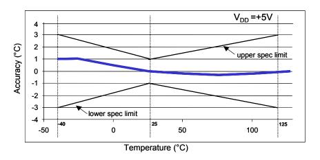
Figure 2. aTS51 Accuracy Range vs Temperature
