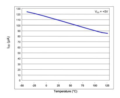
Figure 3. aTS51 Current vs Temperature
