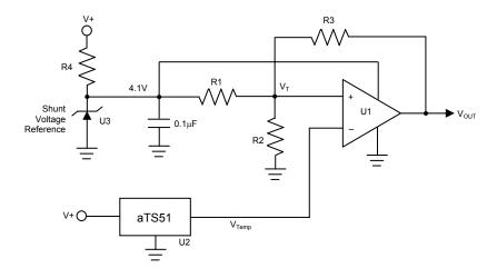
Figure 6. Thermostat/Fan Controller
