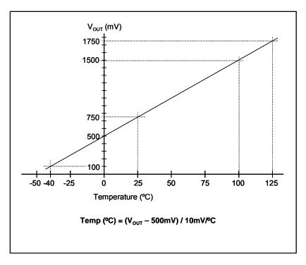
Figure 1. aTS51 Output Voltage vs. Temperature
