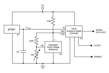
Figure 4. Serial Output Temperature to Digital Converter (Full Scale = +125°C)
